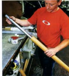
12: Each reconditioned stanchion is individually packed and despatched back to the customer by City Link. Turnaround on the whole job is usually no more than one week.
