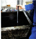
7: Recesses at the stanchion ends, such as those machined for fork bushes, have to be protected from the chroming process, so the tubes are wax dipped at the ends and dressed back to ensure only the bearing surface receives the new chrome.
