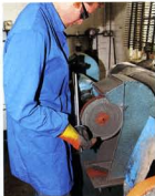
6: Before chroming, the ground surface is finished off and checked. Any remaining pits means the stanchion goes back to the grinder.
