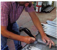
2: Before work commences, the stanchions are engraved internally with the customer reference, so there's no danger of your fork tubes getting mixed up with anyone else's.
