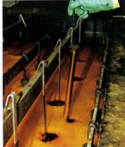
8: The industrial hard-chroming process deposits new metal onto the stanchion surface. The material gives a durable surface which, in many cases, is more resistant to pitting than some factory finishes.
