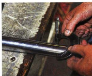
3: Measuring the stanchion on an unworn section gives a reference dimension to work to for reconditioning. All figures are cross-referenced against existing records to double check.
