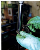
9: The tubes are chromed oversize to ensure there's enough new metal to be ground down to size.
