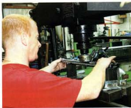
4: Next step is to check the stanchions for truth. Even undamaged forks can show slight bending due to the braking forces encountered in several years hard use. Bent forks are straightened in the press before proceeding.
