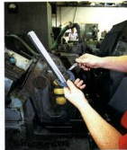
11: The final check. The reconditioned stanchions should be correct to factory tolerances, and are frequently better than standard.
