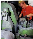
10: Then it's back to the grinder to machine the new surface. Accurate setting up means the centreless grinder can machine the finish to very close tolerances.
