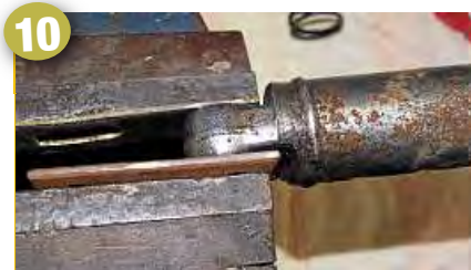
Protect the axle boss with packer pieces
