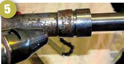
5 Apply some heat before dismantling
