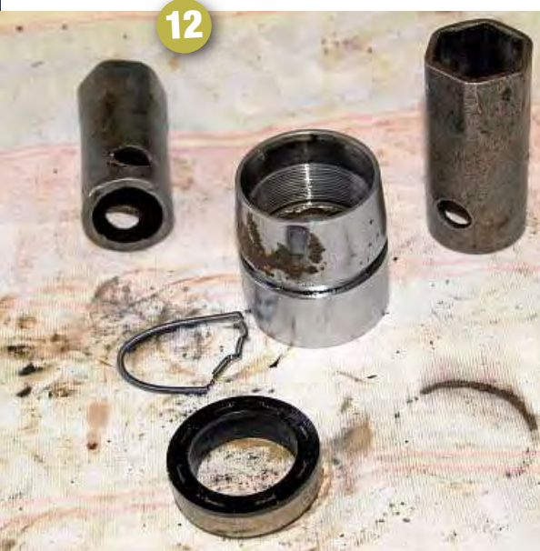
Seal evicted with extreme prejudice... and a simple box spanner
