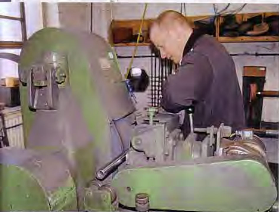
Old chrome is removed on a centreless grinder
